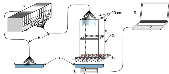
Figure 1: Experimental set-up: a. Water container, b. silicone tubes, c. multichannel dispenser, d. PMMA (poly(methyl methacrylate)) cube ( $\theta_0 = (65.2 \pm 2.9)^\circ$ ), e. coated grate, f. digital balance, and g. computer
