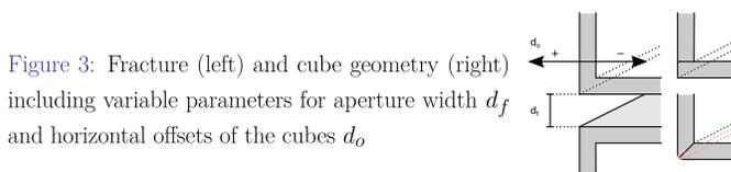
Figure 3: Fracture (left) and cube geometry (right) including variable parameters for aperture width  $d_f$  and horizontal offsets of the cubes  $d_o$
